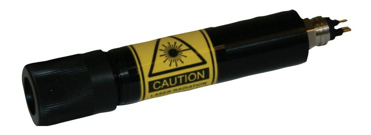
The laser module is a category II low power red laser. The laser can be powered from an 8-30VDC supply and is equipped with over voltage and reverse polarity protection. Standard units are supplied in a durable hard anodised aluminium housing and are depth-rated to 3000m. When used in pairs, imagery scaling is possible by mounting the lasers a set distance apart to identify targets at an equivalent spacing.
