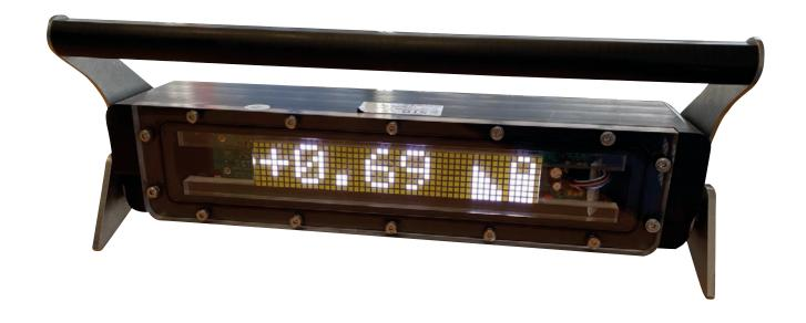
The STR SeaLevel combines our high visibility SeaText white LED display along with a high accuracy orientation sensor and rechargeable battery pack. It has been engineered for diver deployment but is also well suited for other applications such as ROV deployment. The unit is robust, simple to operate and is highly configurable. When used to measure level, the sensor can be changed from forward facing to upward facing display without further configuration
