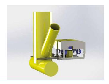
"The system has a number of tangible benefits. Importantly, there is no need to clean away marine growth build up from the members prior to the survey, with the result that the readings are fast and reliable. Operators can get a reading and a status report within seconds. This makes the SeaGamma technique particularly cost effective."
