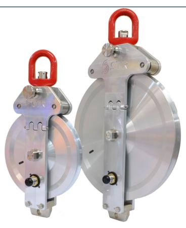
The STR SeaCount is our latest generation of cable measurement system, replacing the previous T-Count product line, offering improved performance, accuracy and reliability. The paid-out cable length is shown on an LCD display, on a PC's screen, and can be forwarded as RS232 serial data for use with a wide variety of data logging systems. Typical applications include SideScan Sonar towfish, Sub Bottom Profilers, Remotely Operated Vehicles, CTD systems and Magnetometer arrays.
