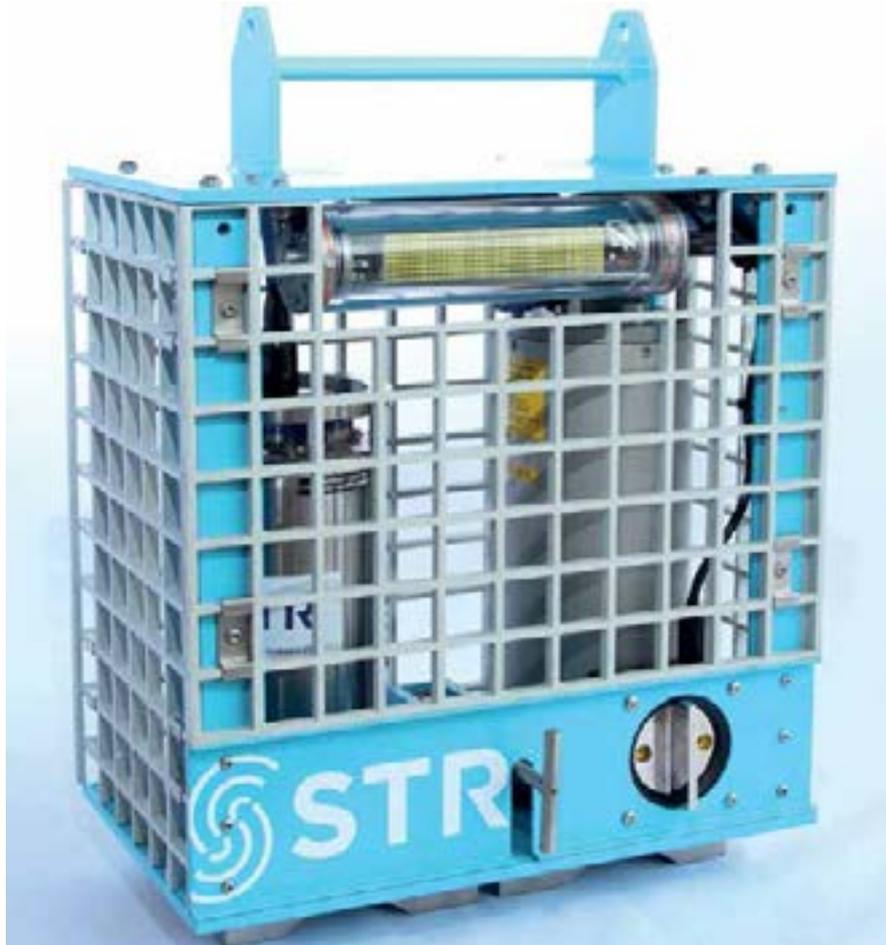
The STR Gyro Frame can be configured to client requirements using either an aluminium or stainless steel frame. All frames are supplied fully certified and come complete with ROV lifting handle, two leg lifting strop and a sacrificial base plate.
