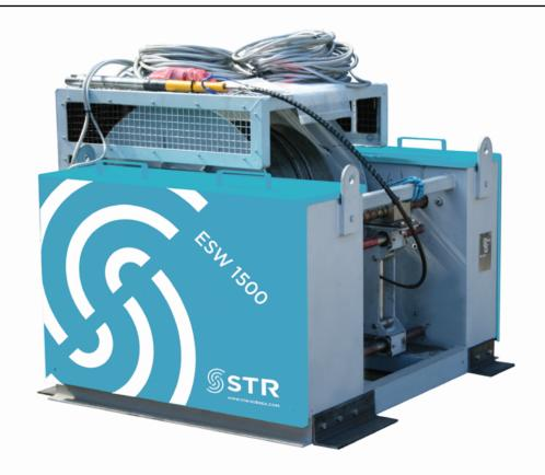
The STR ESW-1500 is a compact electric winch designed for the installation of 1000m of 11.4mm armoured coaxial cable. This model will also accommodate a wide range of electro-optic and umbilical cables.
