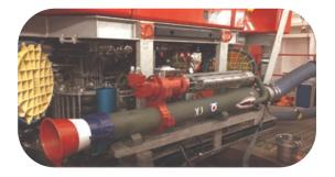
The STS Piranha range is Subsea Tooling Services latest design of high performance dredging equipment. A light weight slim lined dredger designed to fit directly to the side of any work class ROV. The dredger system comes with 360 degree swivel heads which dramatically reduces wear on the ROV manipulator by eliminating all the rotation torque from the suction hose, making dredging much easier and more efficient.
