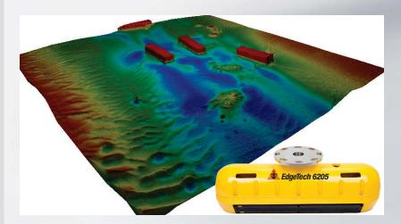
The 6205 uses ten receive element transducers and one discrete transmit element. The high number of channels enables superior rejection of multipath effects, reverberation and acoustic noise commonly encountered in the shallow water survey environment.
