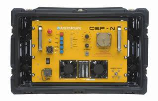
The CSP-N1200 seismic energy source is the driving force behind Applied Acoustics' Dura-Spark range of sound sources that have extremely hard wearing electrode sparker tips. This durability is a consequence of the CSP's reverse polarity high voltage charger and unique proprietary thyristor switching.
